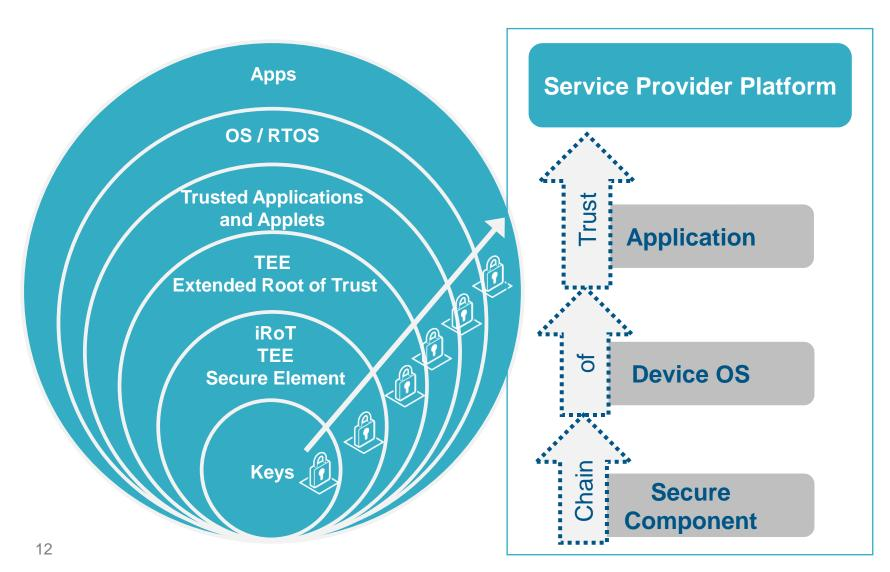
Root of Trust technology within devices enables 'Chains of Trust' to be built. These chains allow device manufacturers and service providers to offer secure digital services while ensuring device integrity and security, alongside end-user privacy.
